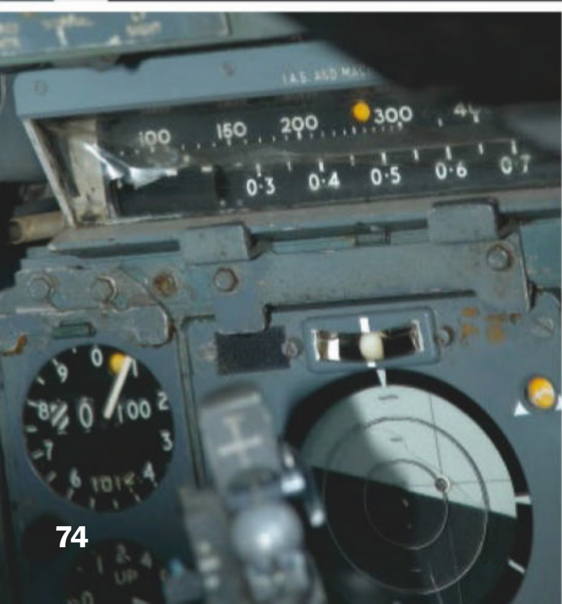
Below: The linear 'strip' speed display that replaced the conventional dial in the F.6
